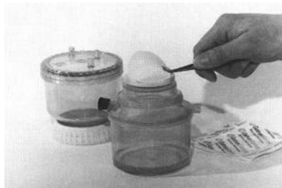
Fig. 18. Placing a sterile membrane filter on the membrane filtration unit.
