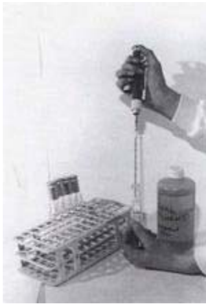
Fig. 13. Adding 1 ml of sample to 9 ml of diluent to make a 1:10 dilution of the sample.
