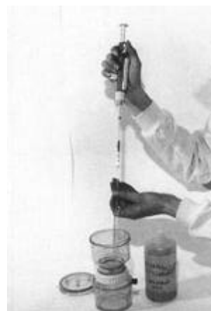
Fig. 20. Adding 5 ml of sample to the membrane filtration unit.
