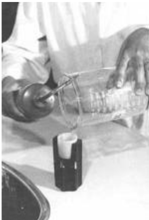
Fig. 3. Washing the sides of the container with dilute detergent solution.
