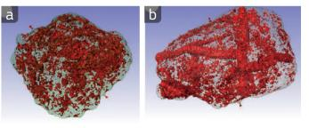
... X-ray microtomography images of soil aggregates (~ 2 mm in size), from (a) cropland and (b) grassland. The pores, in red, where microorganisms live and develop, are small and fragmented in cropland aggregates. They are larger in grasslands due to the higher presence of roots. (MME)
