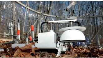
Soil respiration chambers are used to measure  $\mathrm{CO}_{\mathrm{2}}$  emissions by soil organisms. (ORNL)
