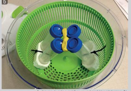
.... It is easy to make a centrifuge, you just need  $({\bf a})$  a salad spinner,  $({\bf b})$  two styrofoam bases with two holes each, and four tubes. (ALE, SMM)
