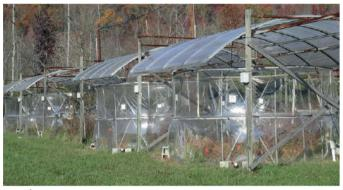
In Tennessee (USA), special chambers are constructed in order to manipulate CO<sub>2</sub> and temperature and register the effects on soil organisms and plants. (PK)
