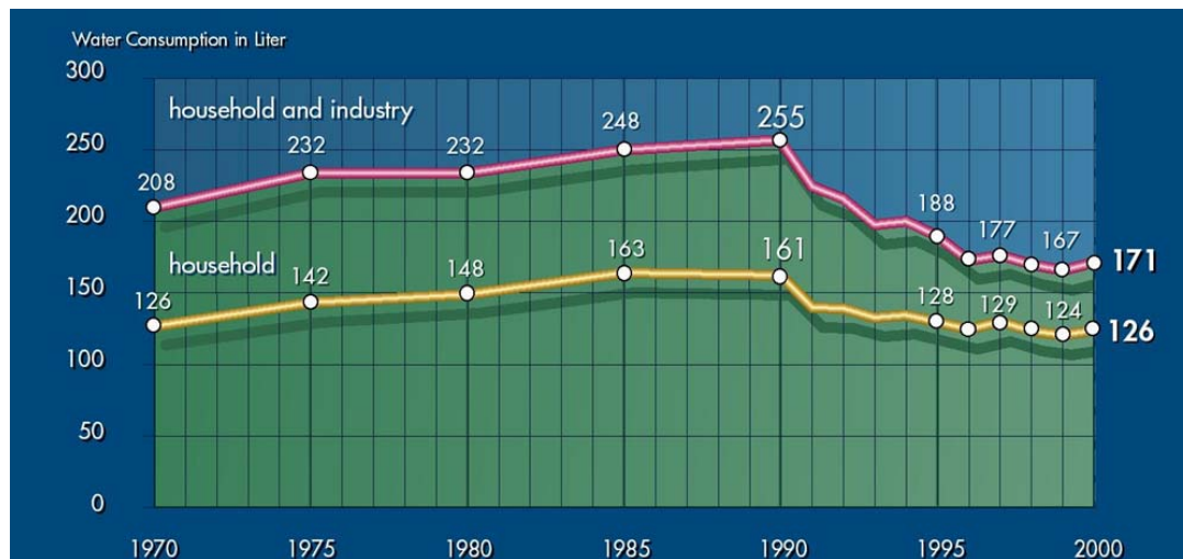
Figure 2: Water consumption in household and industry in liters per day and per capita
