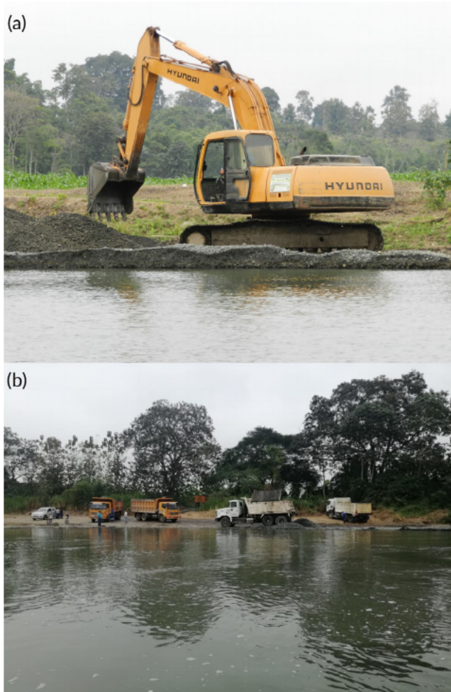
FIGURE 4 Physical destruction of river banks and bottom caused by the removal of gravel for construction. Pictures from the Guayas River basin in western Ecuador
