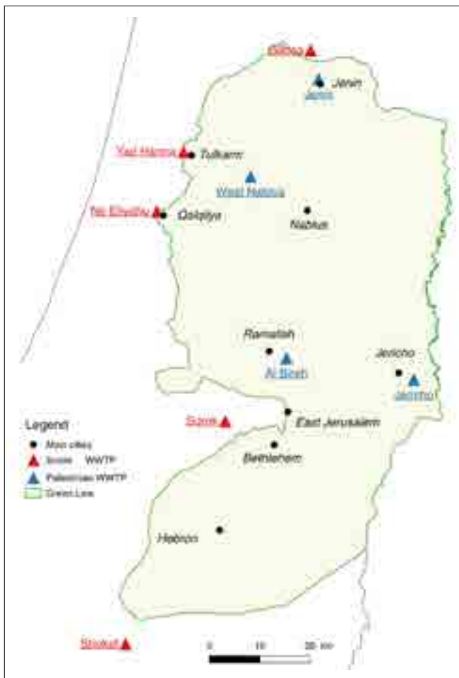
Figure 10-2 Wastewater treatment plants in Israel treating wastewater from the West Bank (Source: authors using QGIS)
