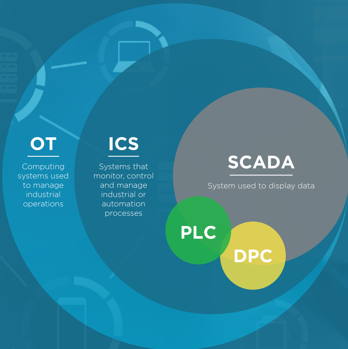
Figure 1: Relationship Between OT, ICS, and SCADA
