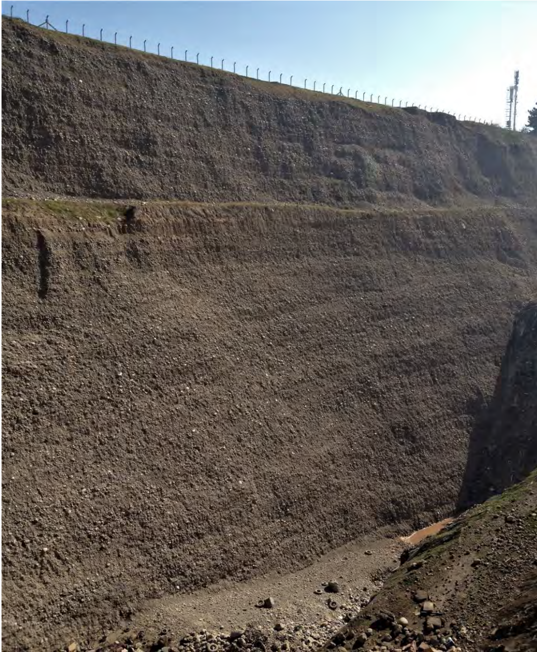
Figure 2. Stratigraphic sequence observed in a gravel pit near the Maipo River, Santiago, Chile, which served as basis for the conceptualization of the numerical simulations. The pit is approximately 80-90 m meters deep.
