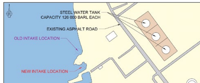
Figure 2: Intake old and new location
